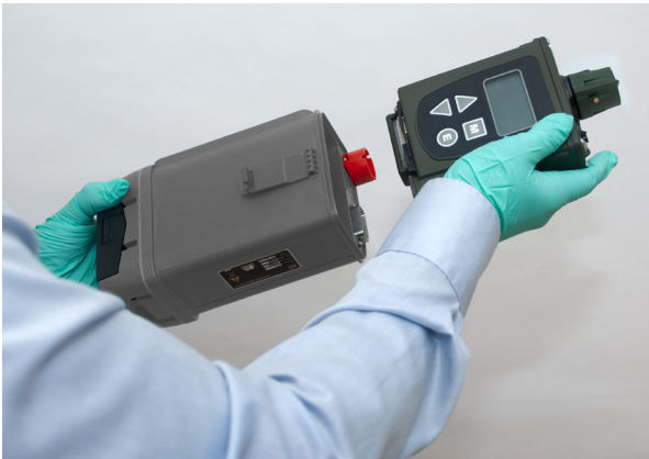
Slide LCD 4 into XID adapter.
